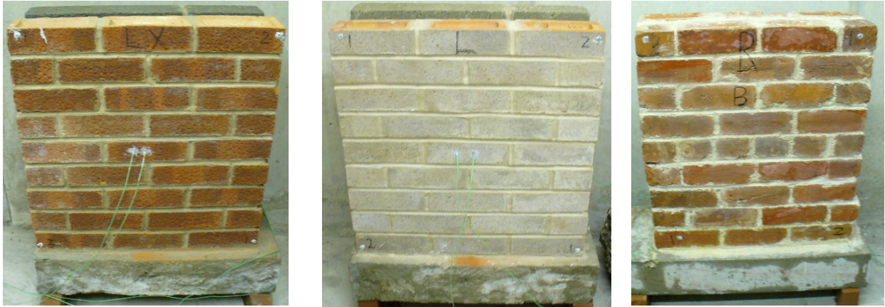
Figure 1: Brick wall panels, from left: London Brick / Breeze Block, Medium Brick / Concrete Block and Reclaimed Victorian Brick
