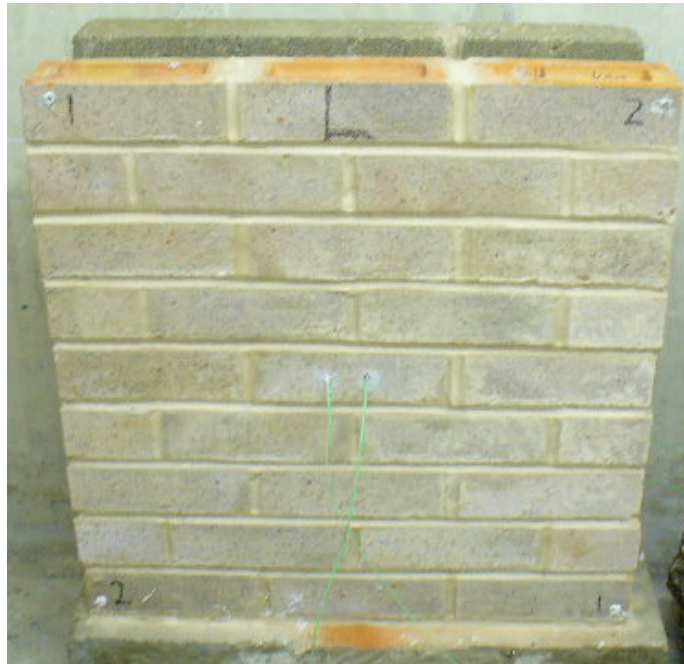
Figure 11: Wall panel L view after drying process - no visible damage
